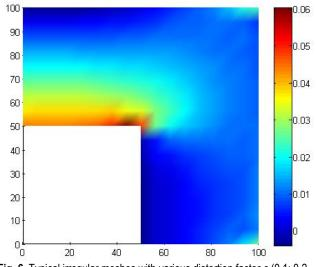
**Fig. 6.** Typical irregular meshes with various distortion factor s (0.1; 0.2 and 0.3) and the normal stress field
