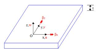
Fig. 1. A plate with positive definition of displacements and rotations
