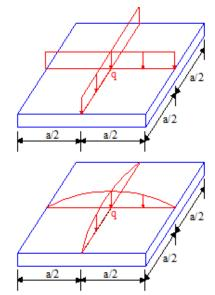
Fig. 7. A clamped square plate under uniformly distributed load and sinusoidal load
