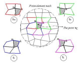
Fig. 2. Schematic sketch of the double interpolation procedure for a quadrilateral element in 2D
