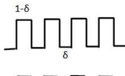
Fig. 2. Clock impulsator with duty cycle equal to 1-δ of time units
