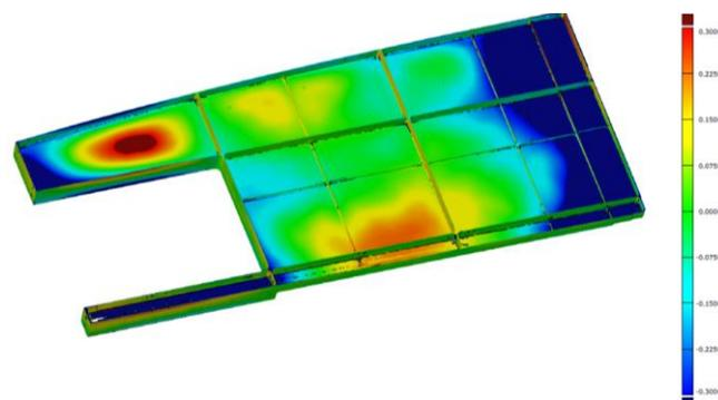
**Fig. 8.** The size of displacements of the beam elements measured by the GOM optical scanning method. The values of displacements reach positive and negative values due to the elastic stresses of the material after HSM treatment. The maximum brown values are due to wall thickness  $< 1 \text{ mm}$  of the pocket between the ribs with a relatively great height – 40 mm. HSM, high-speed machining
