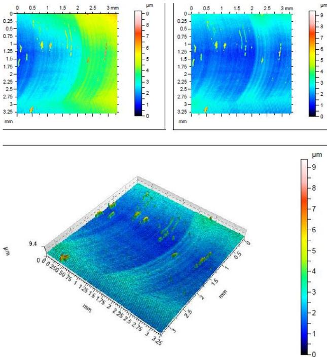
**Fig. 7.** Graphic representation of the roughness of the measured surface,  $S_a = 0.275 \mu\text{m}$  – arithmetic means of discrepancy of the surface’s unevenness from the reference plane: (a) transition area between the machining marks; (b) homogeneous machining area; (c) view of the measurement zone
