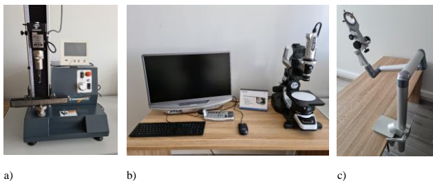
Fig. 3. Test stand: (a) UTM with three-point bending head, (b) digital microscope with mobile head and (c) articulated arm for microscope head
