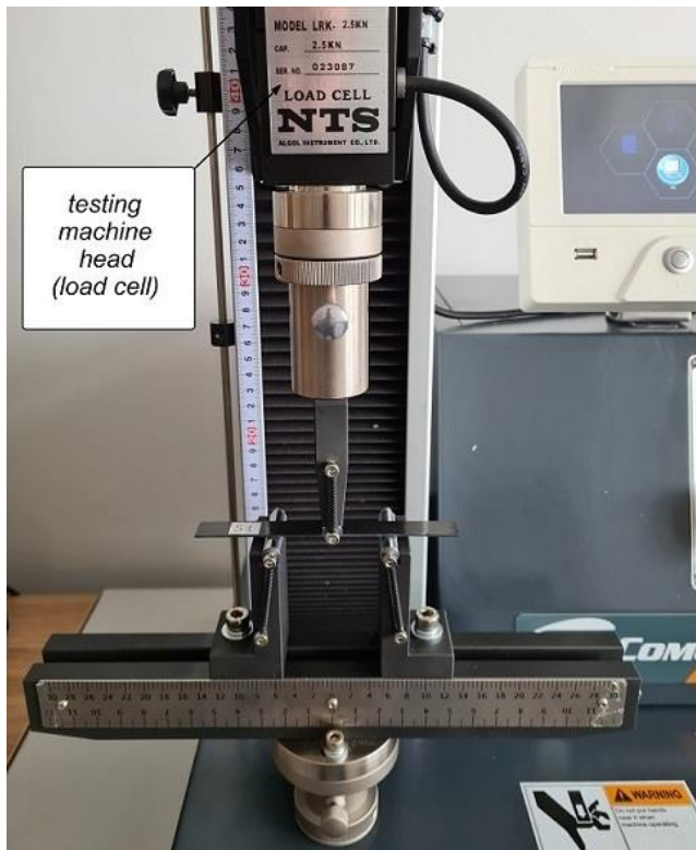
Fig. 8. Test stand prepared for three-point bending tests
