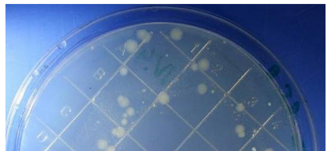
Fig. 6. Section of a CFU plate incubated with MWF. The dots are bacterial colonies that have grown from a single cell. The different sizes of the colonies are due to the different growth rates of the respective bacterial strains and indicates the presence of different species in the sample
