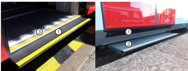
Fig. 3. Extendable steps on the vehicle 14Ev from Škoda Transportation: 1 – movable step; 2 – additional step; 3 – boarding area of the vehicle
