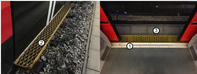
Fig. 2. Fixed step in the railway vehicle Talent of Bombardier Transportation: 1 – boarding area of the vehicle; 2 – fixed step; 3 – platform
