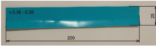
Fig. 3.1. Specimen of LDPE foil used in the tensile test
