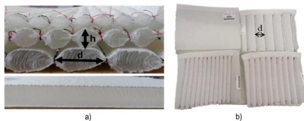
Fig. 2 Spacer fabric variations for experimental testing: (a) cross view, (b) top view; h cushion height, d seam distance
