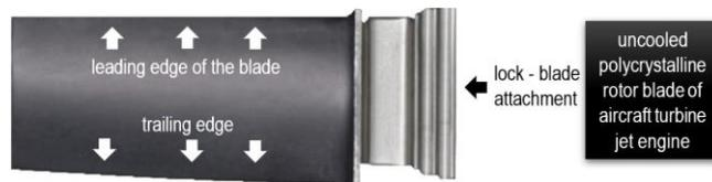
Fig. 1. Example of blade convex (suction face) surfaces
